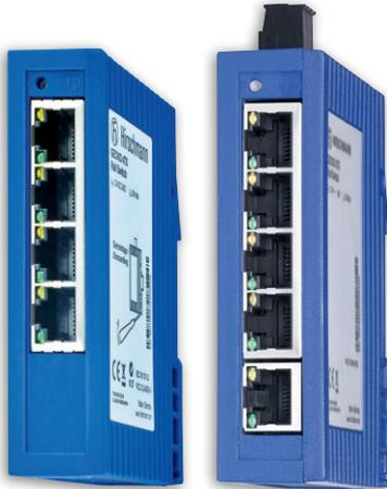
Featuring four or five Fast Ethernet ports (10/100 Mbit/s) and the ability to mount on a DIN rail, the compact dimensions (25 x 114 x 79 mm) of the GECKO switches require little space and in-active ports can be disabled to protect against possible misuse.
