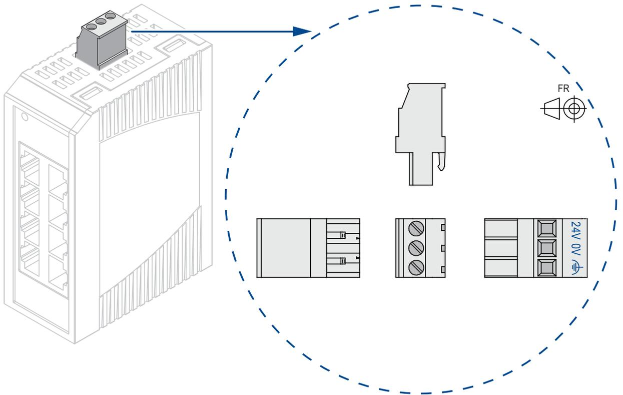
Figure 2: 3-pin terminal block, characteristic value HH
