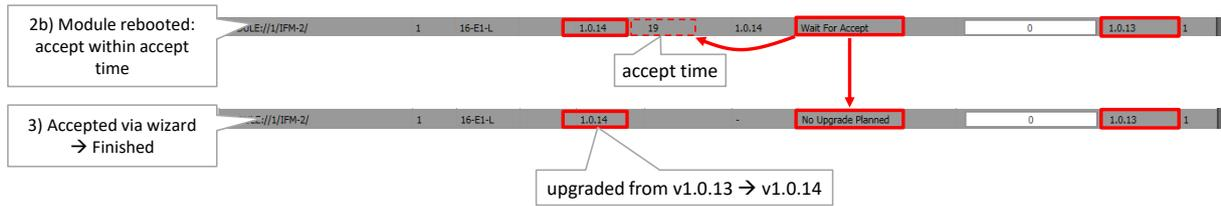
**Figure 105 Step3: Accept Firmware**
