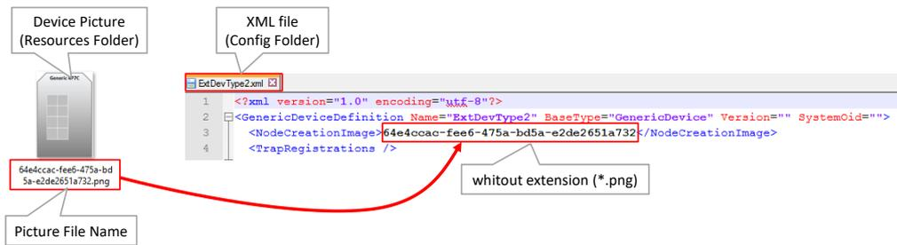
Figure 175 External Device Picture In XML File
