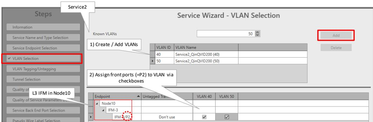
**Figure 84 Multi VLAN/QinQ Service2: Add/Create VLANs and Assign Front Ports**
