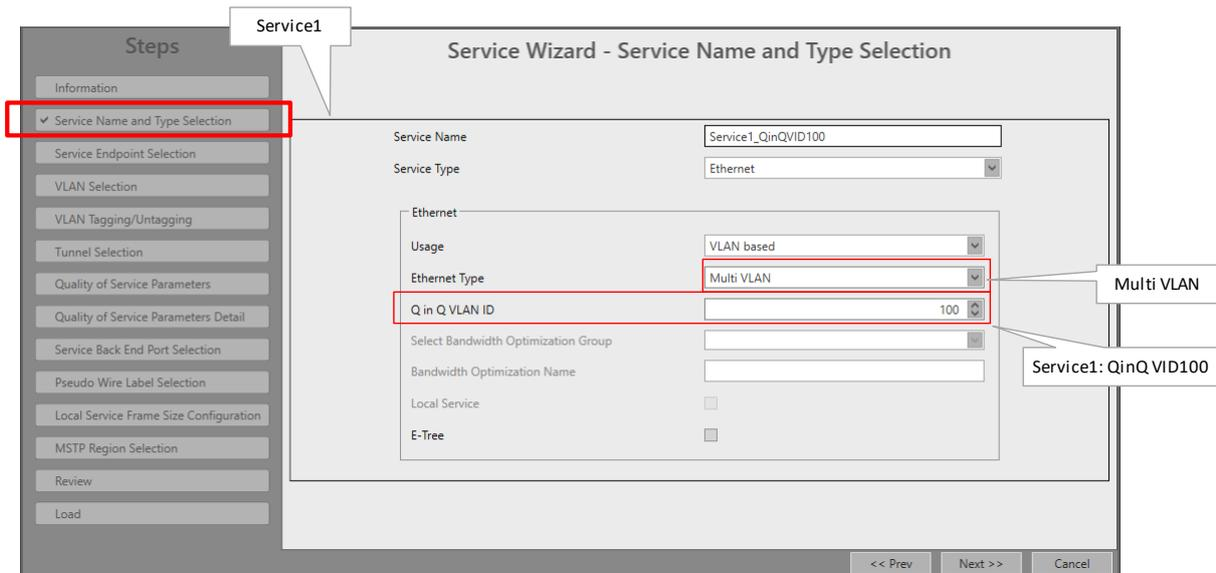
**Figure 81 Multi VLAN/QinQ Service1: Start Creation/Define QinQ VLAN**
