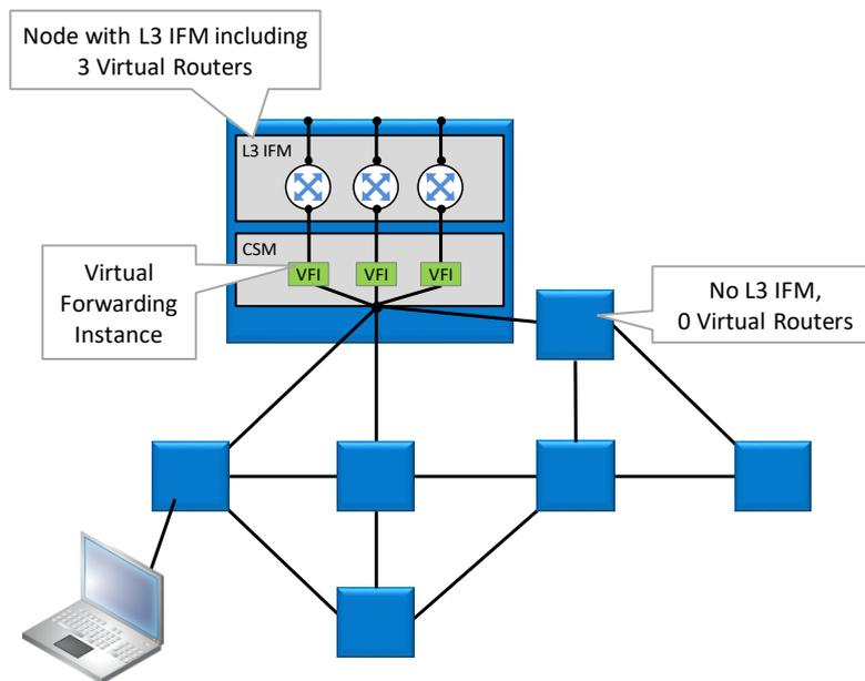
**Figure 116 Virtual Router Example**
