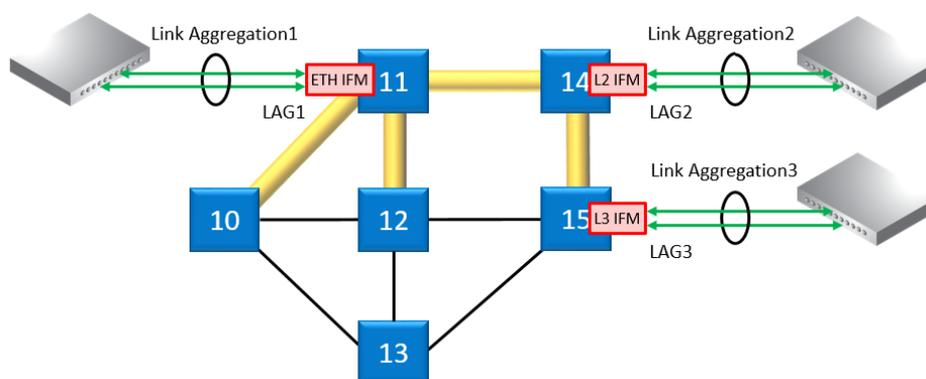
Figure 136 Link Aggregation and LAGs
