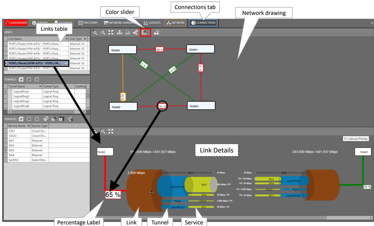
**Figure 26 Connection Tab: Bandwidth Information**
