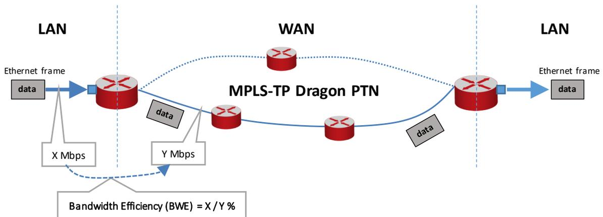
Figure 30 Bandwidth Efficiency
