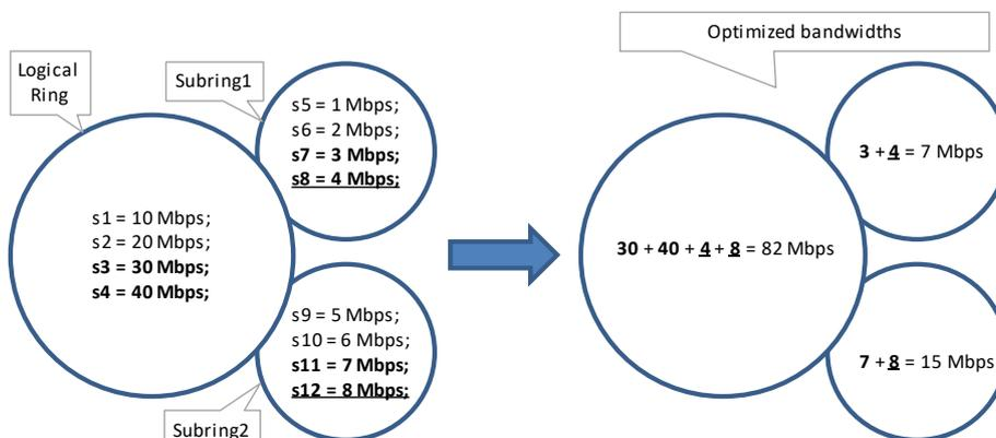
Figure 63 No Interconnecting Service between Logical Ring and Subrings
