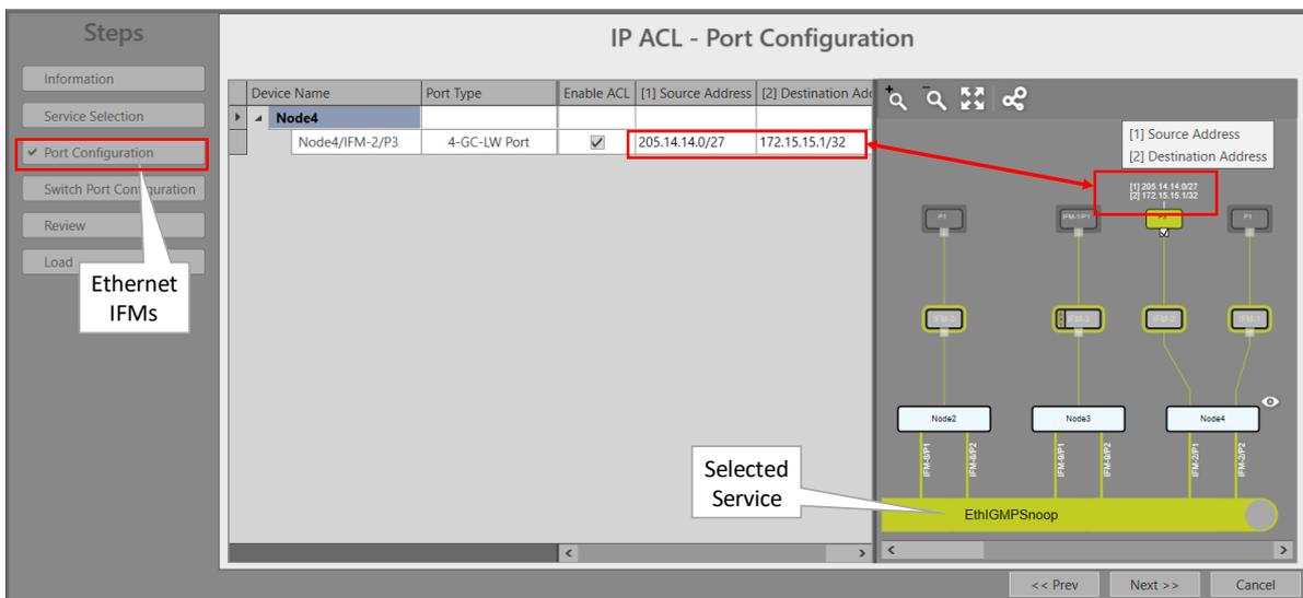
**Figure 131 IP ACL: Port Configuration Example for Ethernet IFMs**
