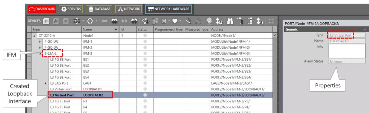
Figure 143 Created Loopback Interface
