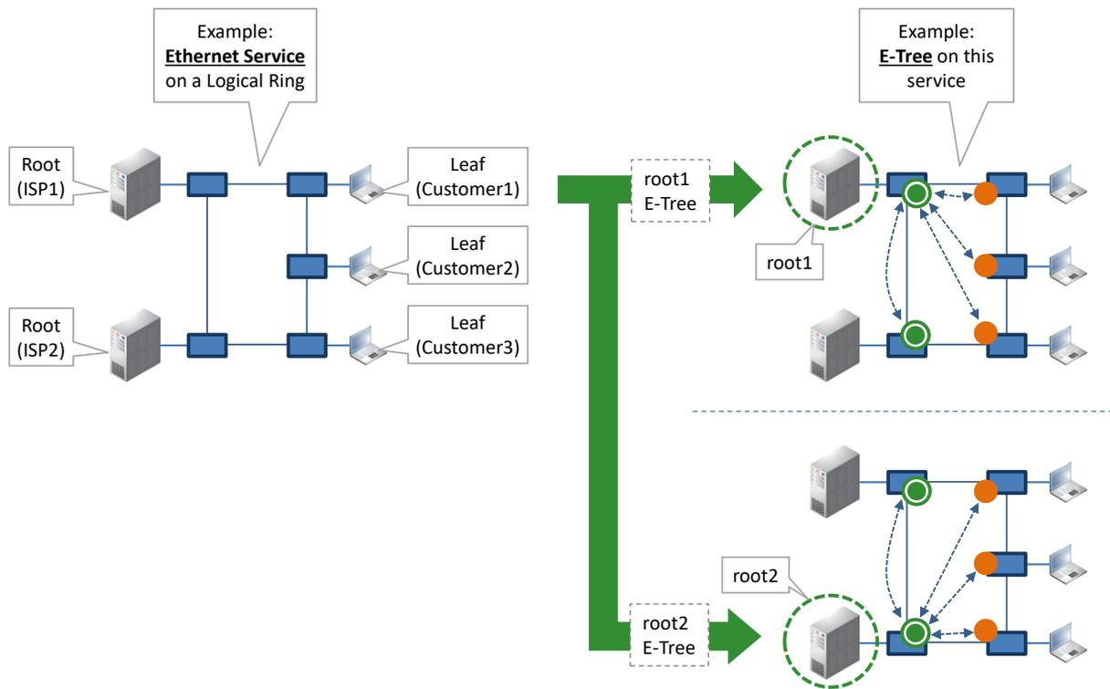
**Figure 2 Example: Ethernet + E-Tree Communication**
