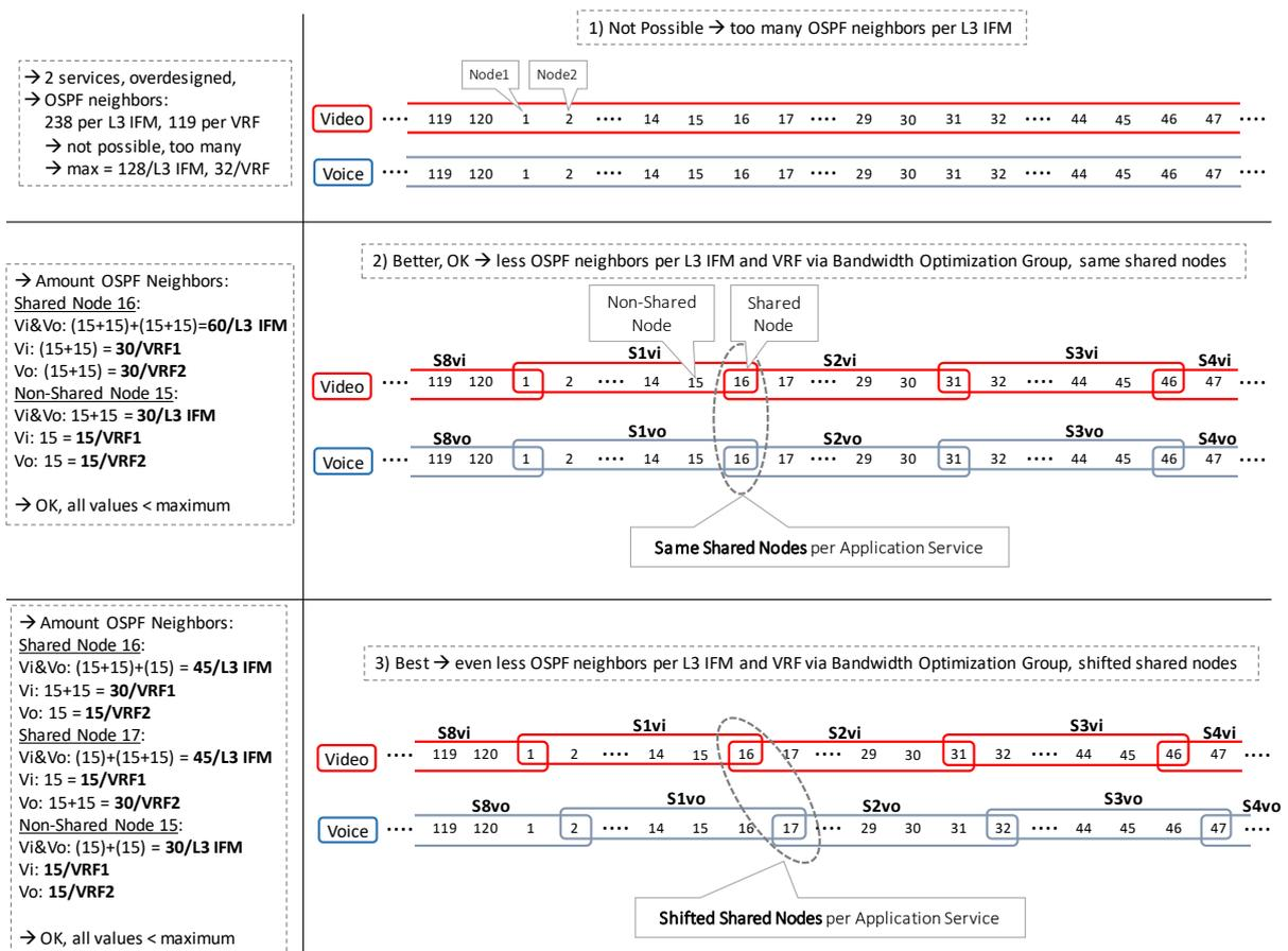
Figure 74 Different Ethernet Service Segmentation Examples
