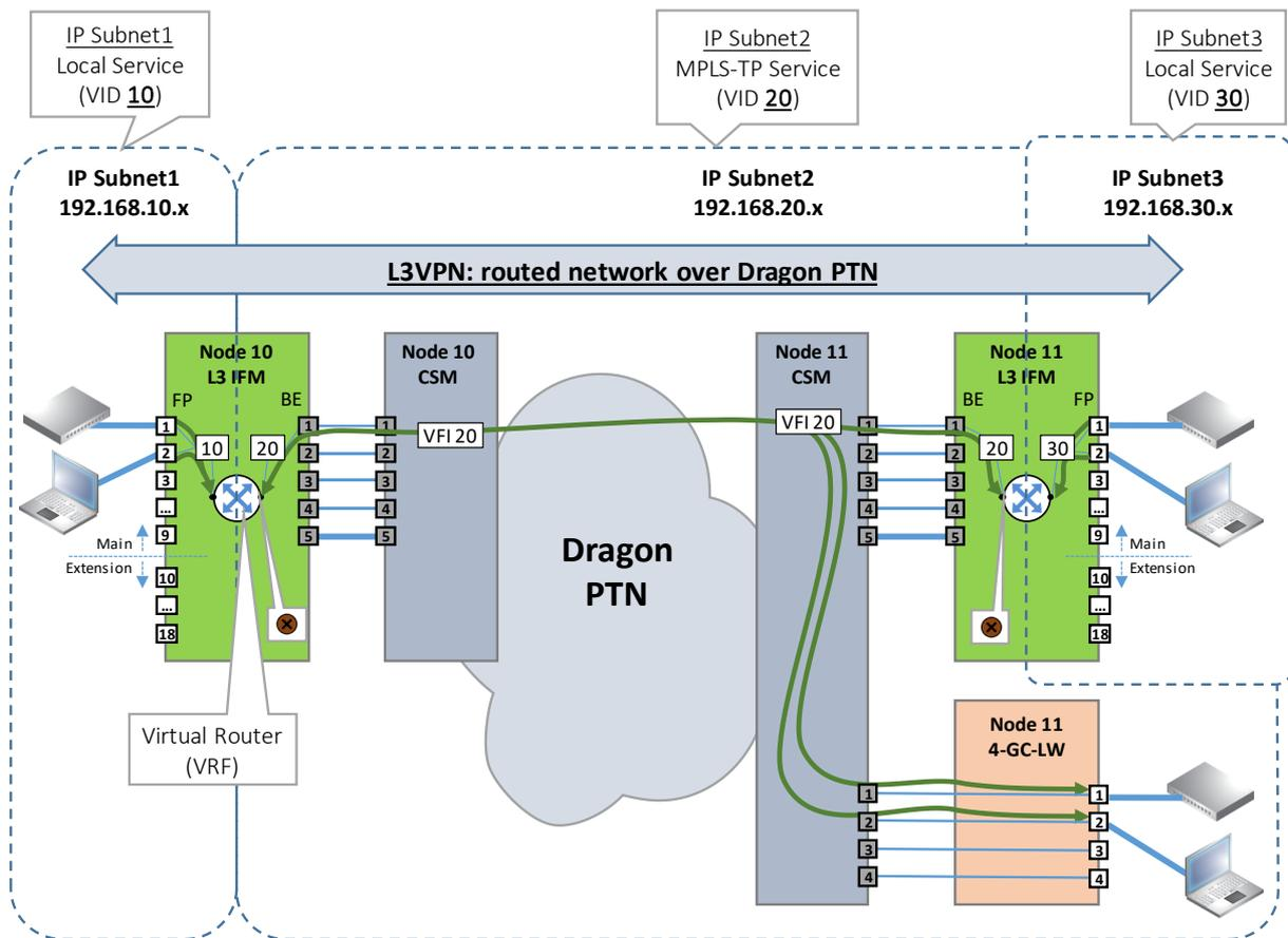
**Figure 86 L3VPN Detailed Example**
