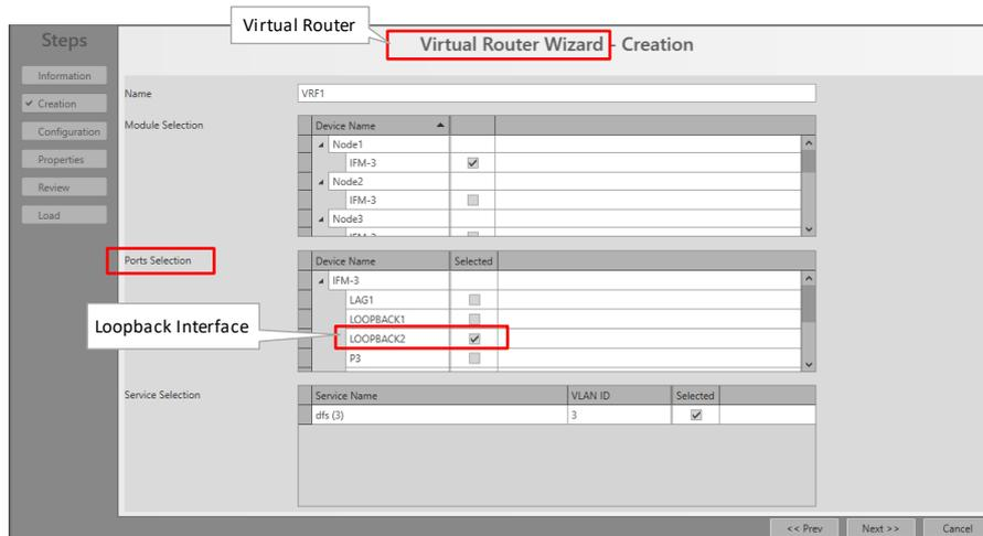
Figure 144 Virtual Router Wizard: Loopback Interface
