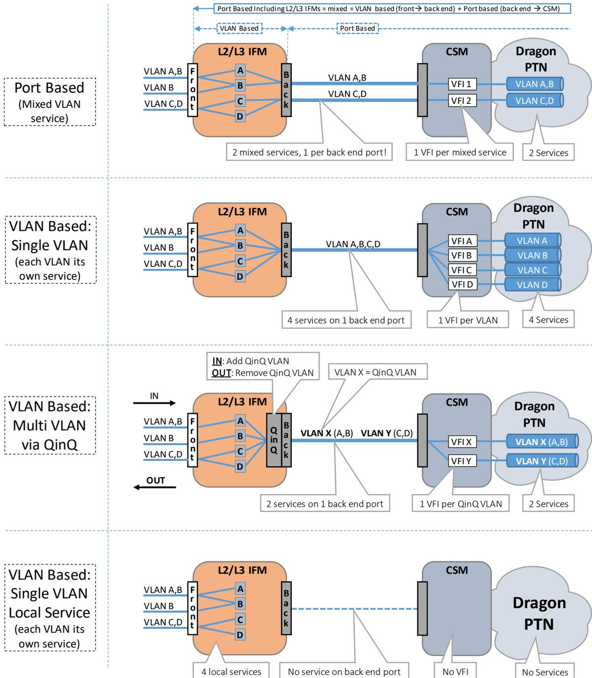
Figure 54 Ethernet Services Examples Overview in L2/L3 IFMs
