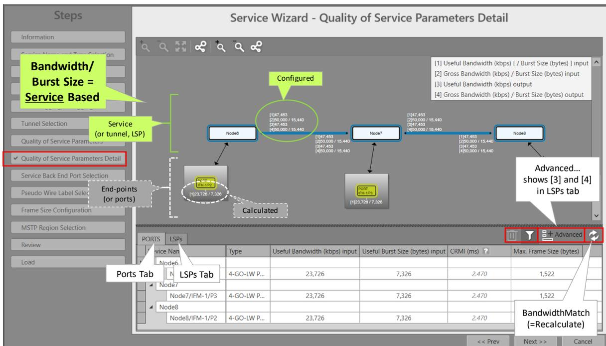
Figure 32 Bandwidth/Burst Size Parameters in Detail
