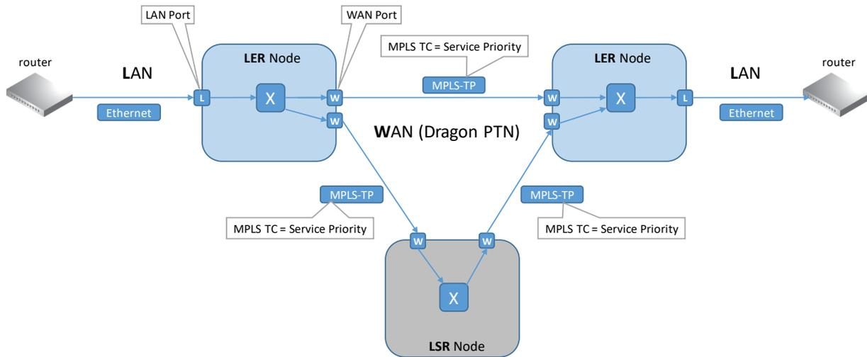
**Figure 47 MPLS TC Mapping (HQoS = Off)**
