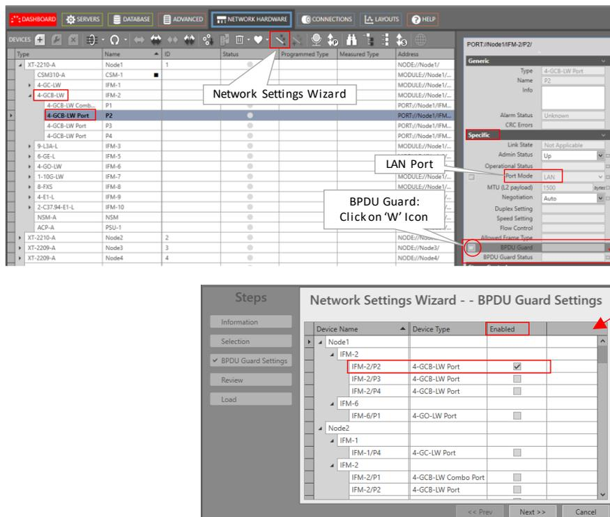
**Figure 4 BPDU Guard on Ethernet LAN Port**
