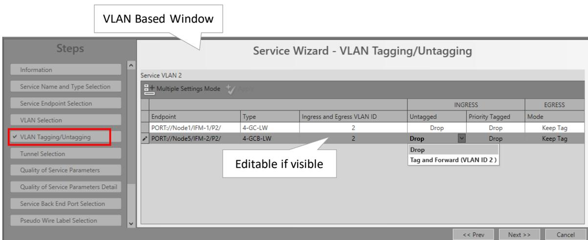
Figure 10 VLAN Based: VLAN Tagging/Untagging
