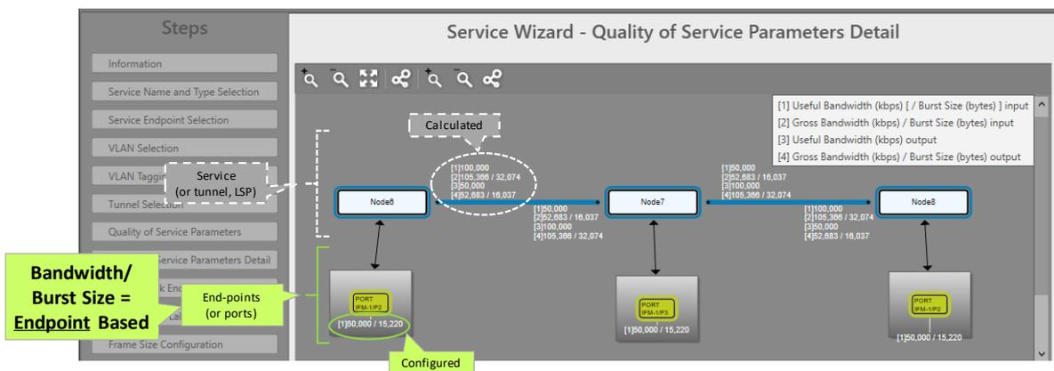
**Figure 37 Bandwidth/Burst Size: Endpoint Based**
