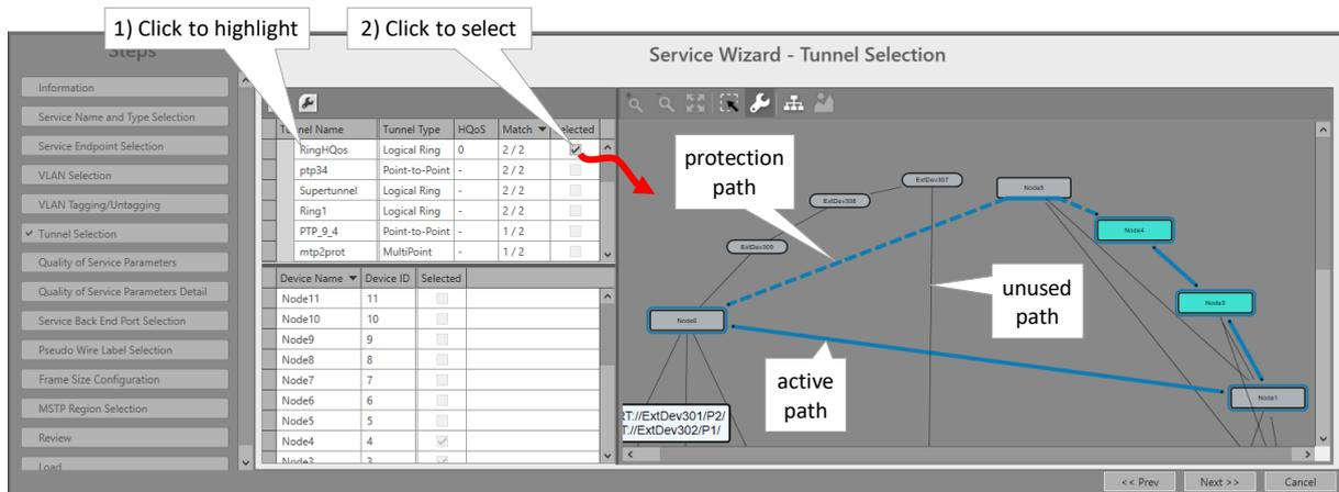
**Figure 12 Selected Highlighted Tunnel**
