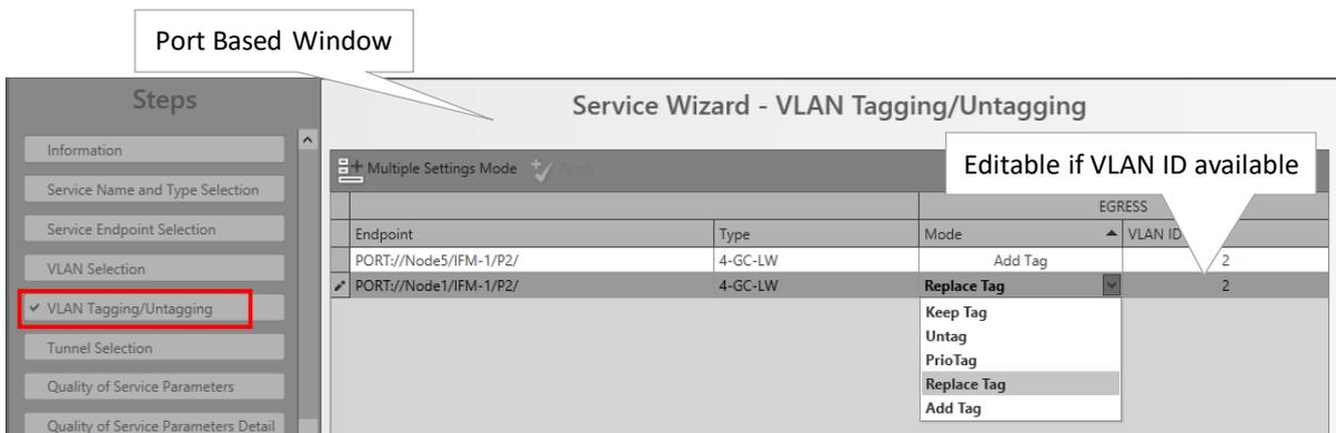
Figure 9 Port Based: VLAN Tagging/Untagging
