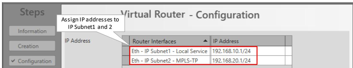
**Figure 88 Assign IP Addresses to IP Subnet1 and 2**
