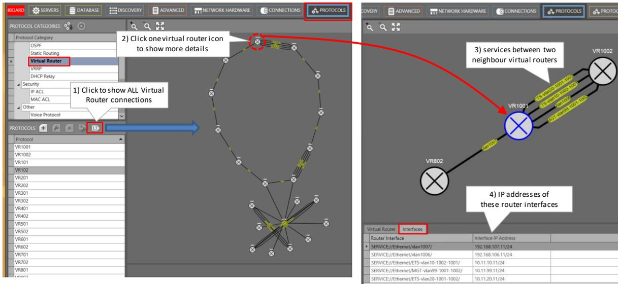
Figure 120 Layer 3 View: Virtual Router Connections Overview
