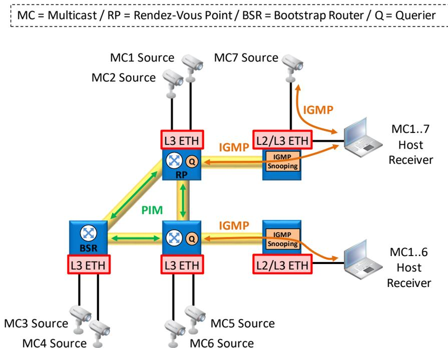
**Figure 100 PIM/IGMP/IGMP Snooping Overview**
