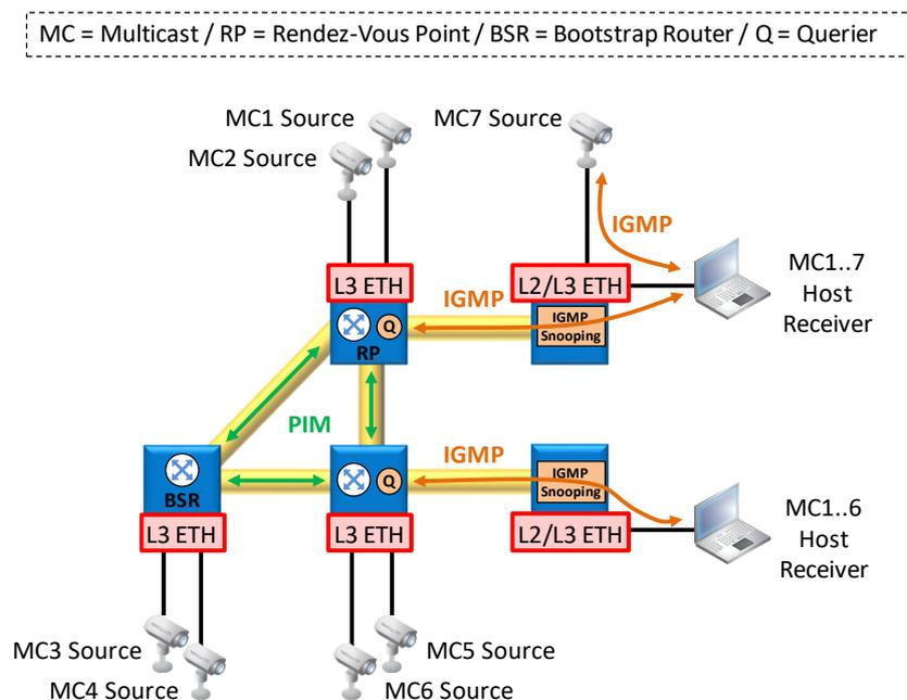
**Figure 106 PIM/IGMP/IGMP Snooping Overview**
