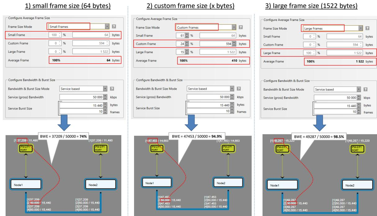
Figure 31 Bandwidth Efficiency Examples in HiProvision
