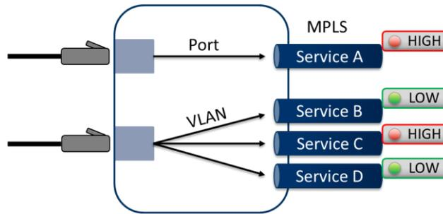
**Figure 21 Dragon PTN Classification: Port Based / VLAN Based**
