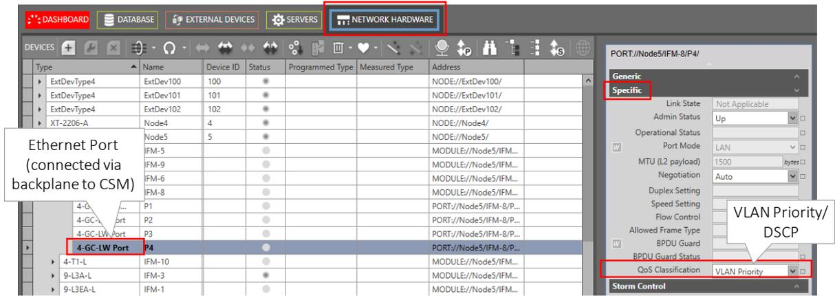
**Figure 46 HQoS = On → QoS Classification: VLAN Priority/DSCP Setting**
