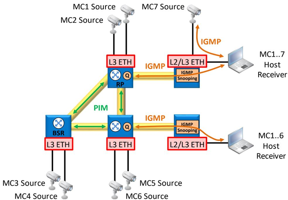
Figure 107 PIM/IGMP/IGMP Snooping Overview
