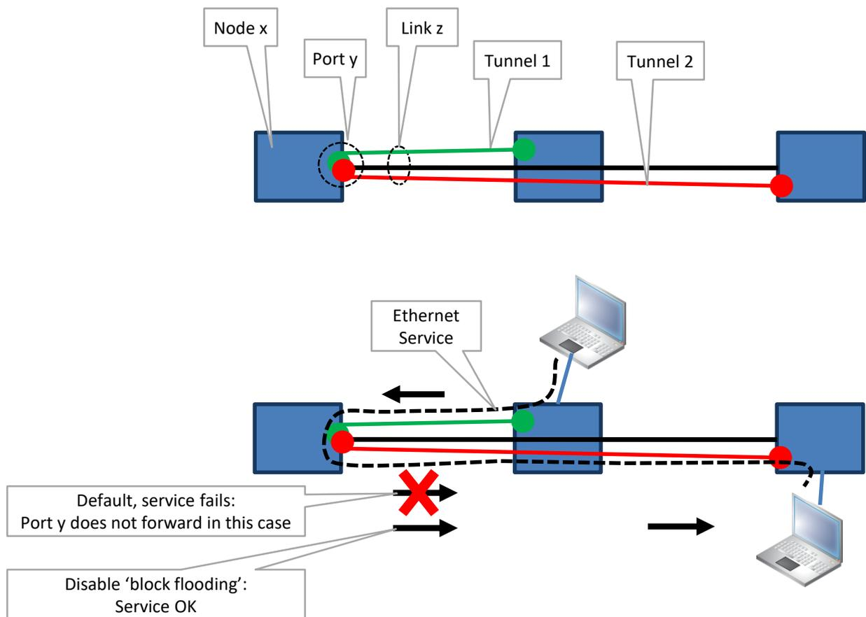
**Figure 16 Ethernet Service Fails with Multiple Tunnels on Same Link**
