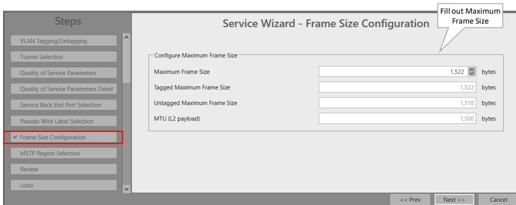
**Figure 14 Frame Size Configuration**
