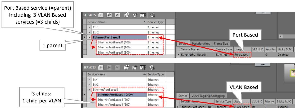
Figure 79 Example-Detailed: Port Based: Created, Result in Services List
