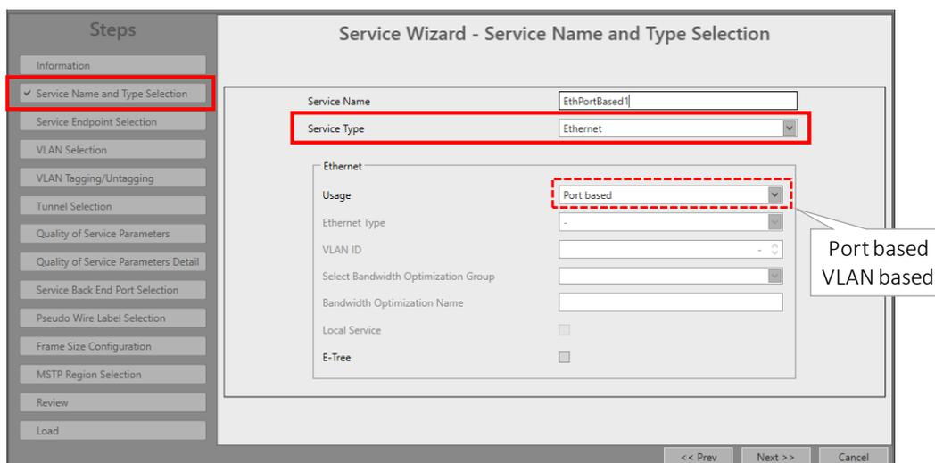
**Figure 5 Service Type: Ethernet**
