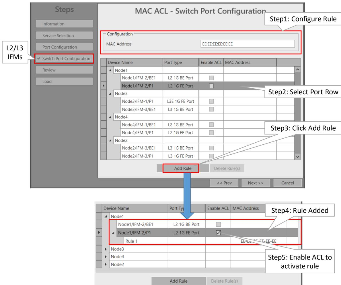
**Figure 134 MAC ACL: Switch Port Configuration Example for L2/L3 IFMs**
