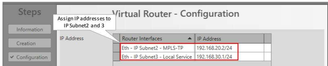
**Figure 90 Assign IP Addresses to IP Subnet2 and 3**
