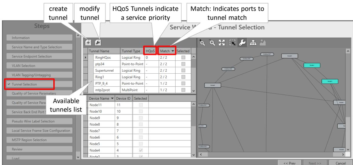
**Figure 11 Ports to Tunnel Match**
