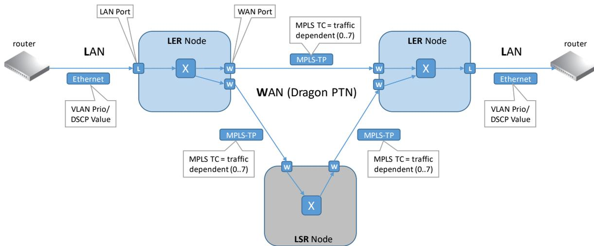
**Figure 48 MPLS TC Mapping (HQoS = On)**
