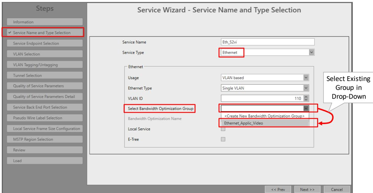
Figure 69 Service Wizard: Assign Service to Existing Bandwidth Optimization Group
