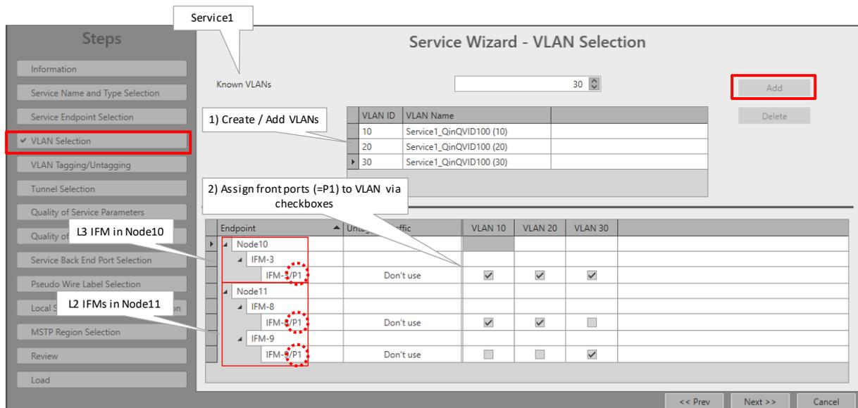
**Figure 82 Multi VLAN/QinQ Service1: Add/Create VLANs and Assign Front Ports**
