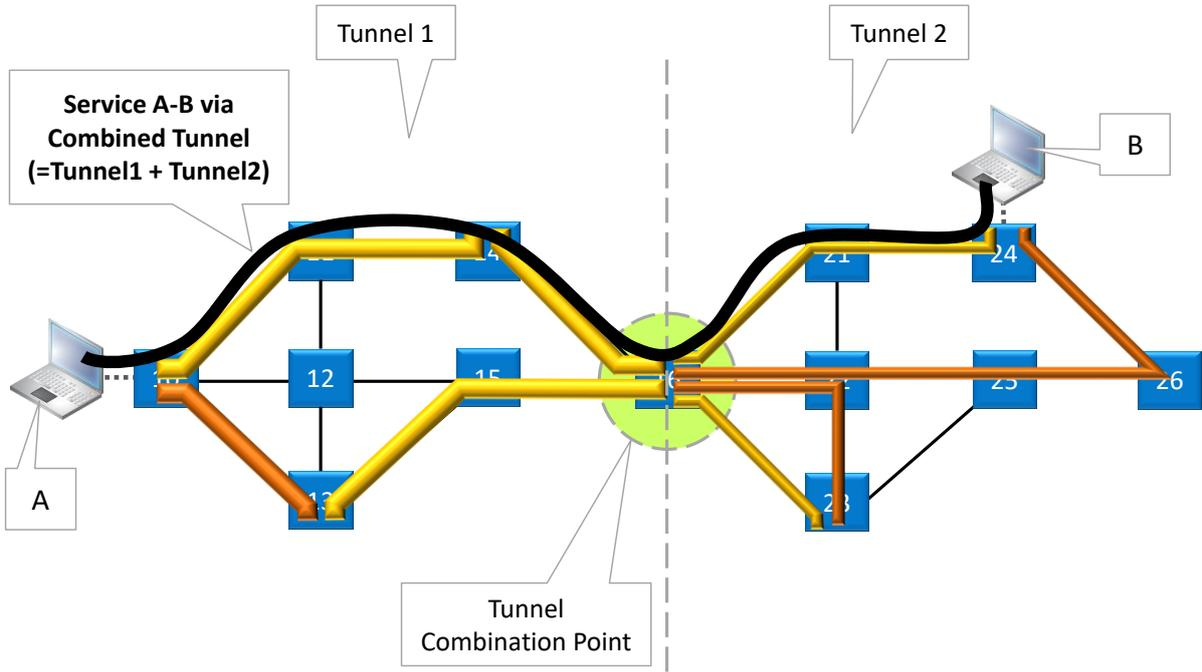
**Figure 3 Service Via Combined Tunnels**
