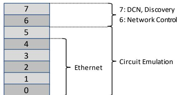
Figure 45 HQoS = Off → Service Priority Mapping
