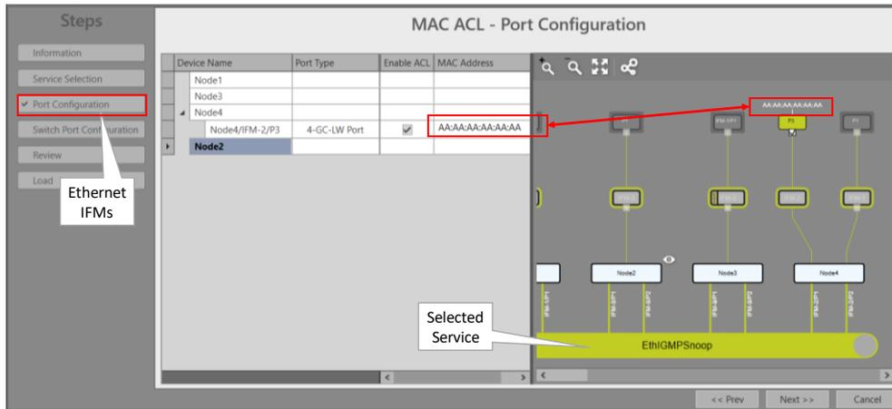
**Figure 133 MAC ACL: Port Configuration Example for Ethernet IFMs**
