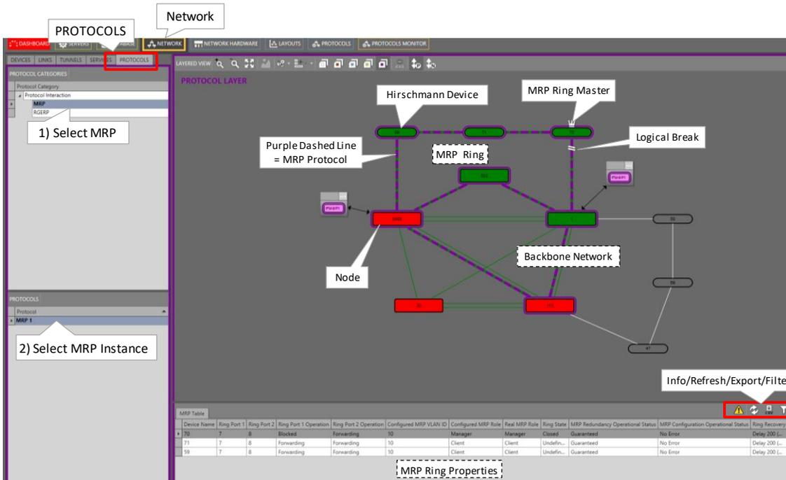
Figure 98 Dashboard → (Monitoring) Network Tile → Protocols Tab
