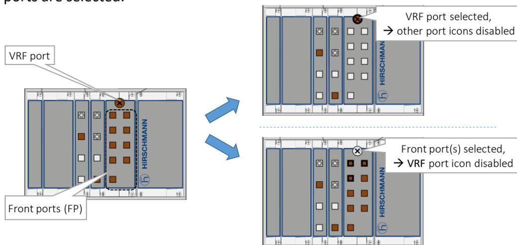
**Figure 56 VRF Port and Front Ports on L3 IFM**
