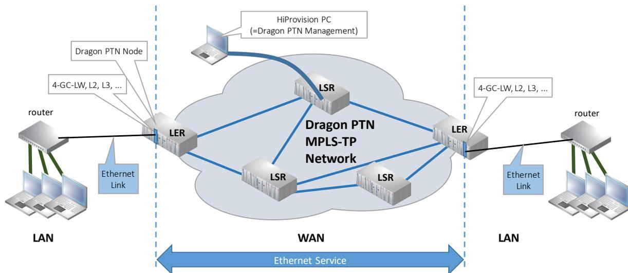
Figure 1 Ethernet Application/Service Example
