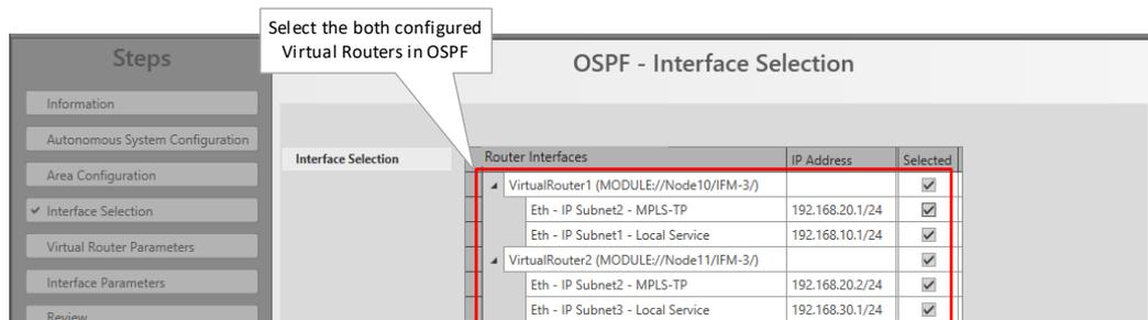
**Figure 91 Configure OSP: Select Both Virtual Routers**
