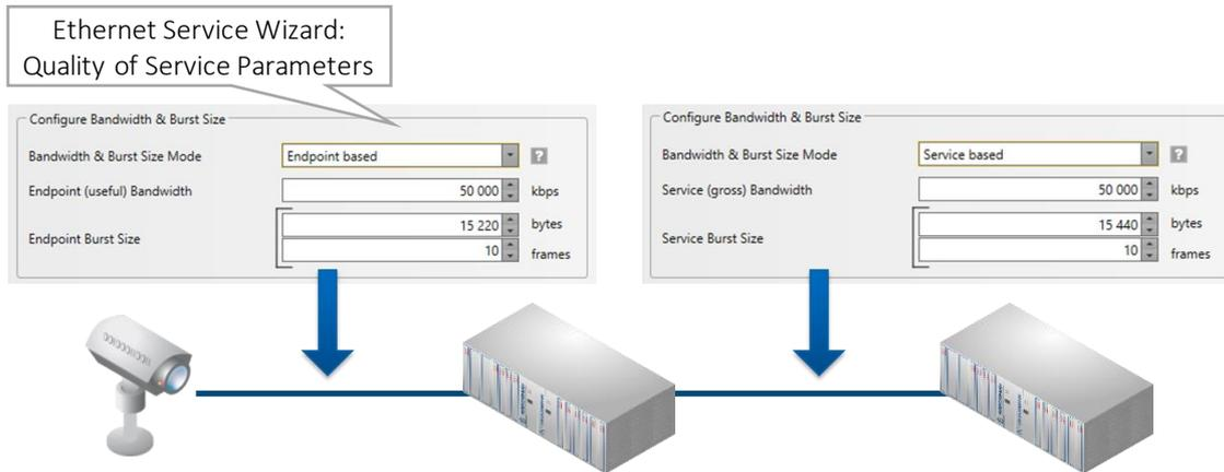
**Figure 23 Bandwidth Profile Configured in the Ethernet Service Wizard**
