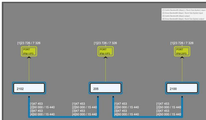
**Figure 24 Resulting Bandwidth Profiling in HiProvision**
