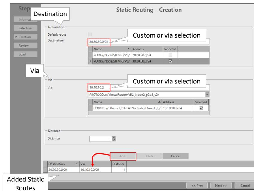
**Figure 114 Static Routing - Creation**
