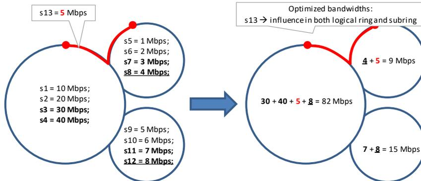
Figure 66 Interconnecting Service S13 Has Influence In Both Logical Ring and Subring
