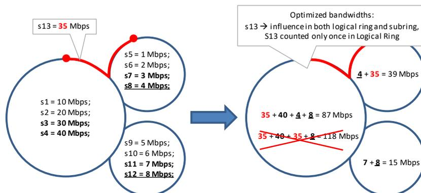
Figure 67 Interconnecting Service S13 Top 2 Highest Bandwidths in Logical Ring
