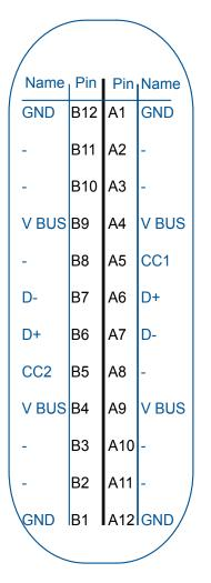
Figure 1: Pin assignment of the USB-C interface
