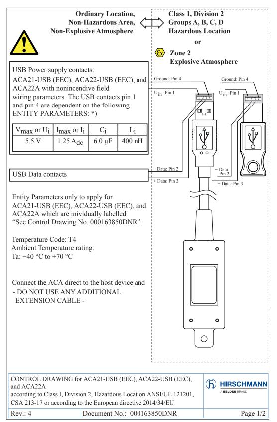
Make sure that the Entity Parameters of the host device meet the following requirements: \*)
