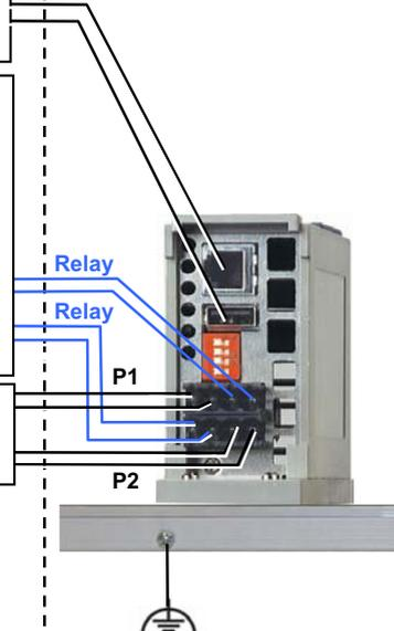
The earth conductor must be at least the same wire size (mm<sup>2</sup> or AWG) as the supply conductors.
