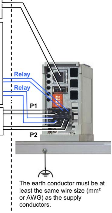
The earth conductor must be at least the same wire size (mm<sup>2</sup> or AWG) as the supply conductors.
