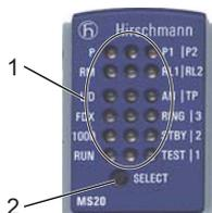
Figure 18: "SELECT" button on the MICE basic modules
