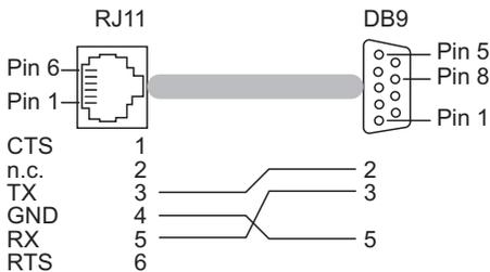
Figure 19: Pin assignment of the V24 interface
