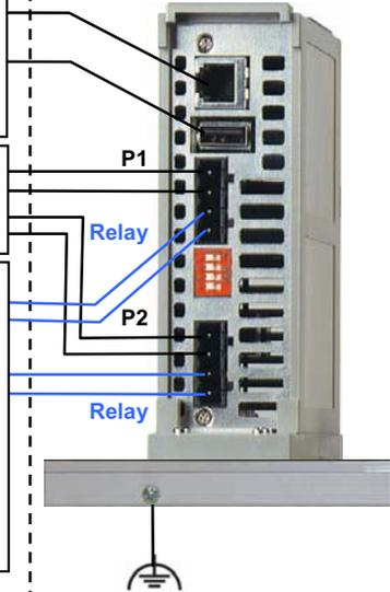
The earth conductor must be at least the same wire size (mm<sup>2</sup> or AWG) as the supply conductors.
