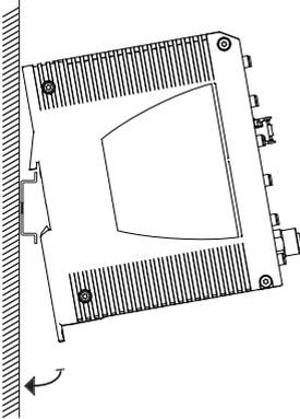
To mount the device onto a horizontally mounted 35 mm DIN rail according to DIN EN 60715, proceed as follows:
