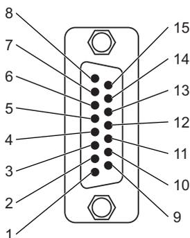
Figure 10: Pin assignment of an AUI interface
