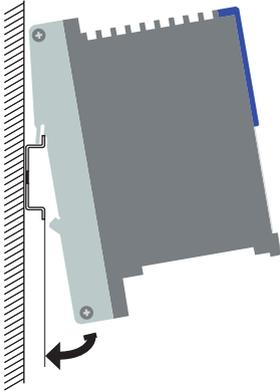
The lower panel of the device casing is grounded via the DIN rail and optionally by means of the separate ground screw.
