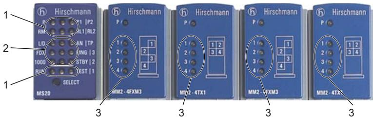
Figure 11: Display elements on MS20/MS30
