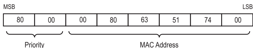
Figure 6: Bridge identifier, example (values in hexadecimal notation)
