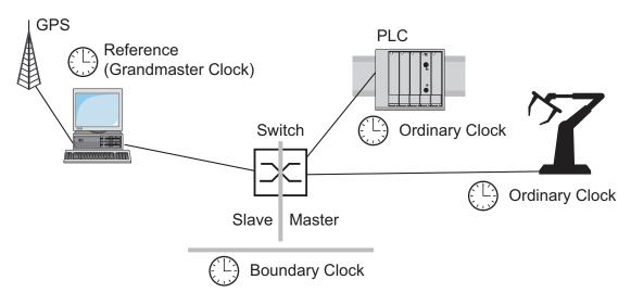
Figure 30: Position of the boundary clock in a network
