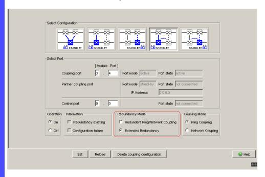
Figure 40: Two-Switch coupling with control line: Selecting the redundancy mode
