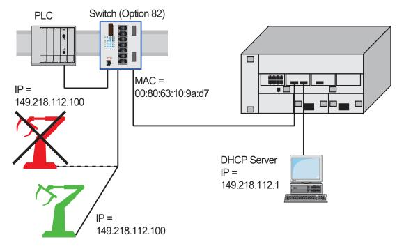
Figure 76: Application example of using Option 82
