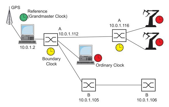
Figure 32: Example of PTP synchronization
