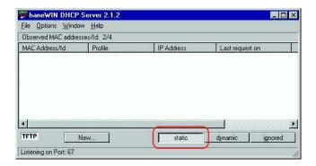
Figure 67: Static address input
