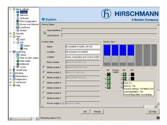
Figure 2: Web-based user interface of the device with tooltip.
