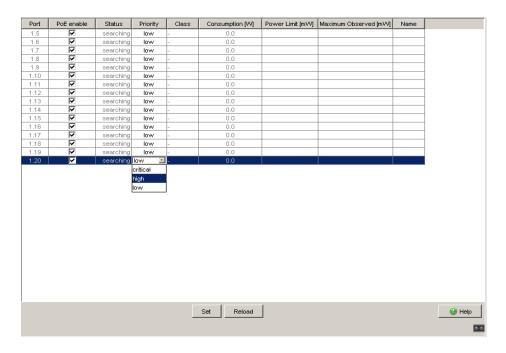
Figure 12: Power over Ethernet Plus Dialog:Port
