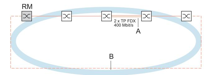
Figure 6: Example of a HIPER-Ring / link aggregation combination RM = Ring Manager
