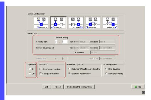
Figure 31: Two-Switch coupling: Selecting the port and enabling/disabling operation
