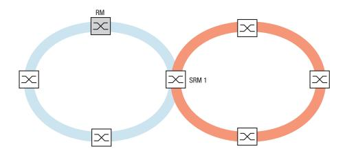
Figure 18: Special case: a Sub-Ring Manager manages both ends of a Sub-Ring at different ports (Single Sub-Ring Manger).
