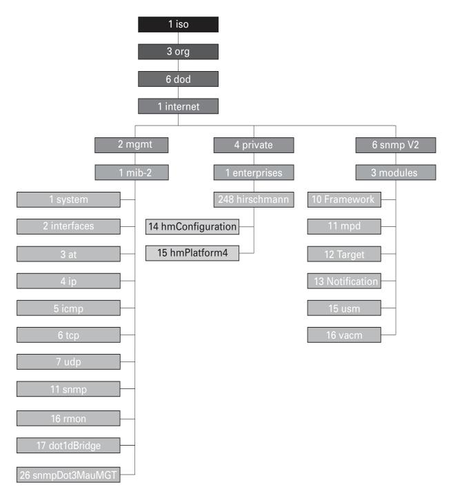
Figure 81: Tree structure of the Hirschmann MIB
