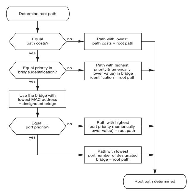
Figure 46: Flow diagram for specifying the root path
