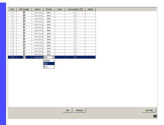
Figure 21: Power over Ethernet Plus, Port dialog (MACH 102 and MACH 104)
