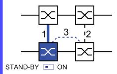
Figure 37: Two-Switch coupling with control line
