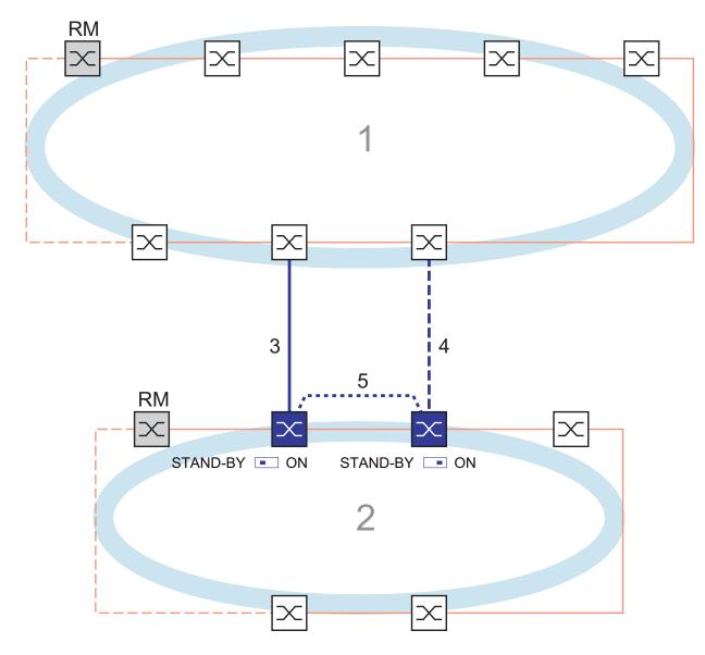
Figure 36: Example of Two-Switch coupling with control line
