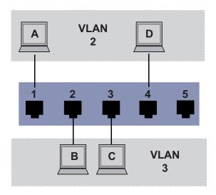
Figure 43: Example of a simple port-based VLAN
