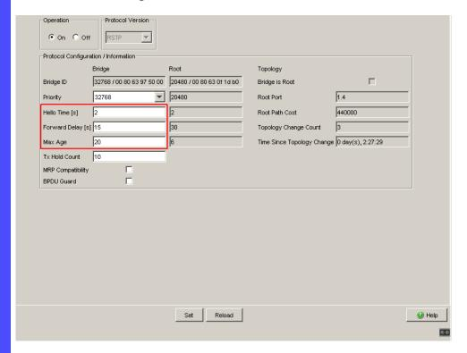
Figure 52: Assigning Hello Time, Forward Delay and Max. Age
