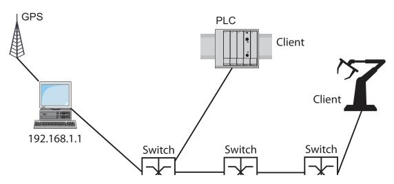
Figure 27: Example of SNTP cascade
