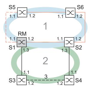
Figure 56: Application example for the combination of RSTP and MRP
