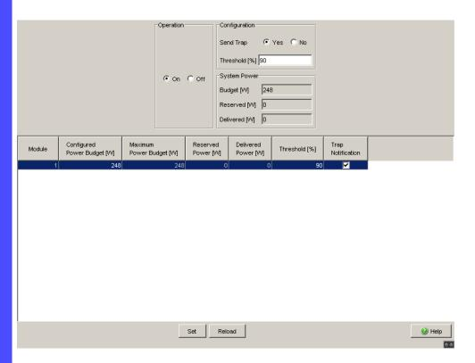
Figure 20: Power over Ethernet Plus, Global dialog (MACH 102 and MACH 104)
