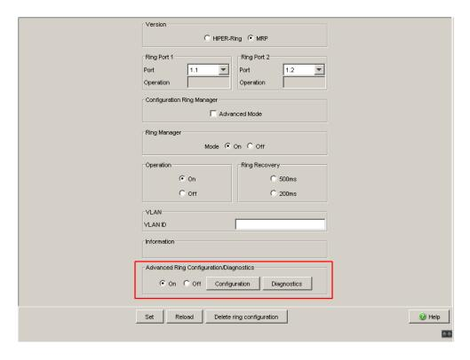
Figure 67: Ring Redundancy Dialog, Advanced Ring Configuration/Diagnostics of an MRP manager.
