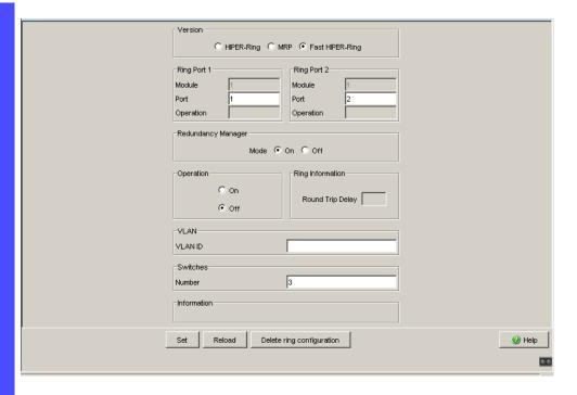
Figure 14: Ring Redundancy dialog (RSR20, RSR30, MACH 1000)
