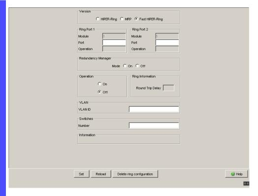
Figure 10: Ring Redundancy dialog (RSR20, RSR30, MACH 1000)
