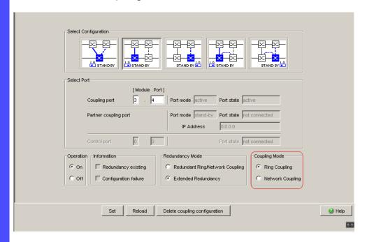
Figure 35: Two-Switch coupling: Selecting the coupling mode
