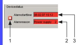
Figure 52: Device status and alarm display
