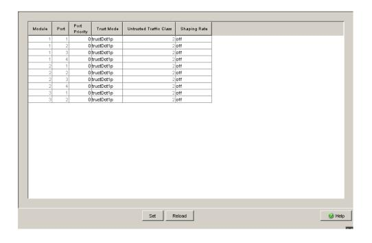
Figure 60: Port configuration dialog for PowerMICE, MACH 104, MACH 1040 and MACH 4000
