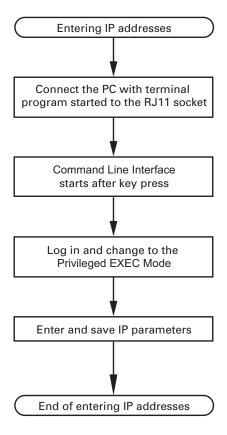
Figure 8: Flow chart for entering IP addresses
