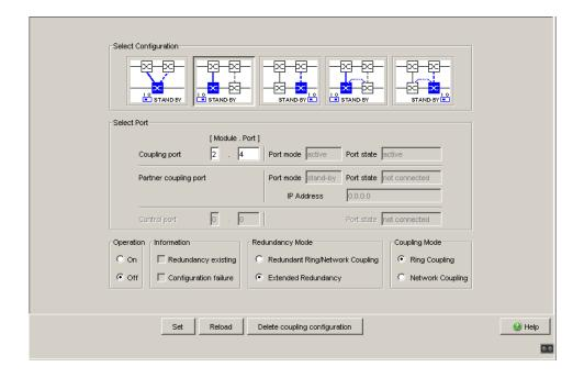
Figure 71: Software configuration of the STAND-BY switch
