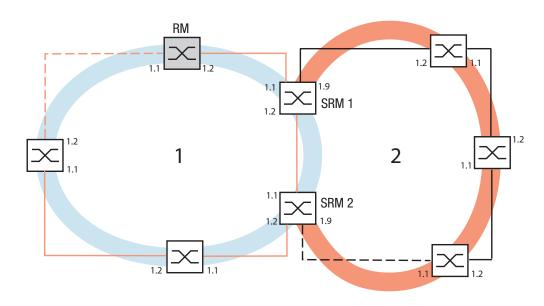
Figure 15: Example of a Sub-Ring structure
