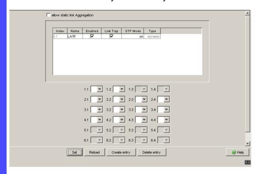
Figure 4: Link aggregation created and named.
