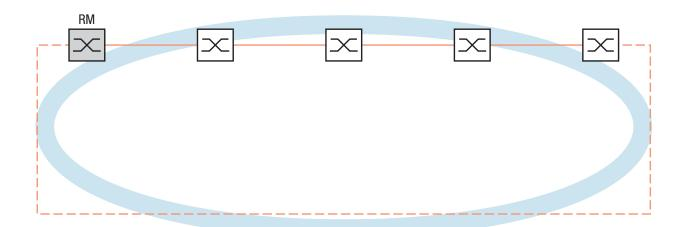
Figure 8: Redundant ring structure
