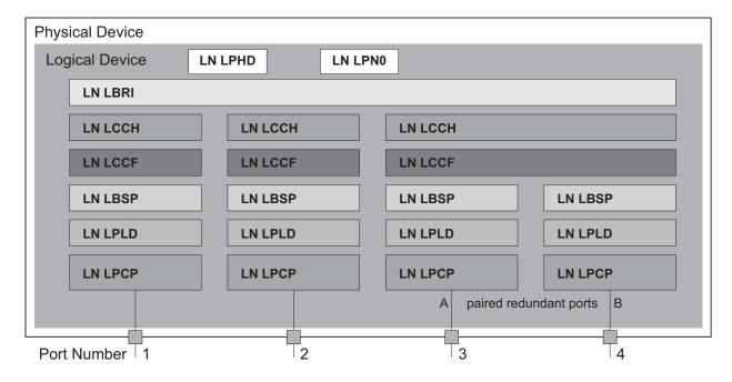
Figure 23: Bridge model based on Technical Report IEC 61850 90-4
