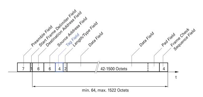
Figure 39: Ethernet data packet with tag
