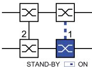
Figure 32: Two-Switch coupling
