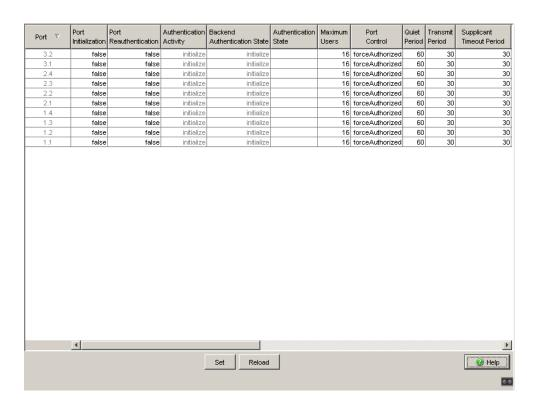
Figure 32: 802.1X Port Configuration Table
