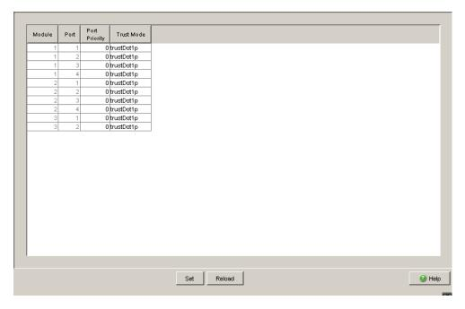
Figure 59: Port configuration dialog for RS20/RS30/RS40, MS20/MS30, RSR20/RSR30, MACH 1000 and OCTOPUS
