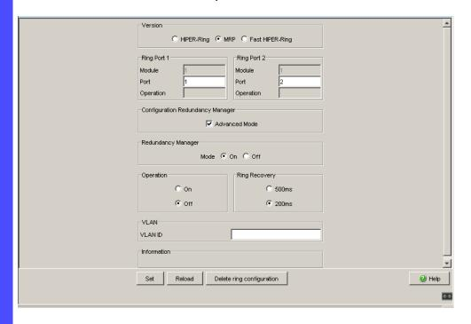
Figure 12: Ring Redundancy dialog (RSR20, RSR30, MACH 1000)
