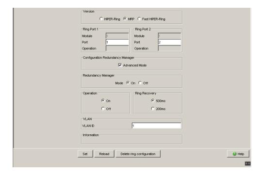
Figure 65: Selecting MRP-Ring version, entering ring ports and enabling/disabling ring manager (RSR20, RSR30, MACH 1000)
