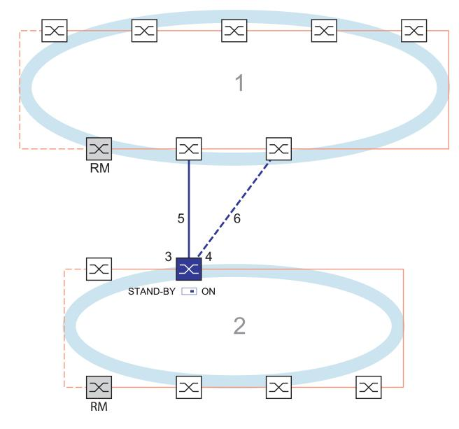
Figure 23: Example of one-Switch coupling
