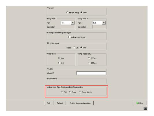
Figure 66: Ring Redundancy Dialog, Advanced Ring Configuration/Diagnostics of an MRP client
