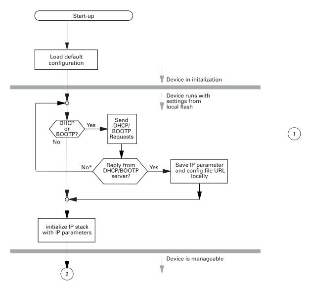
Figure 10: Flow chart for the BOOTP/DHCP process, part 1
