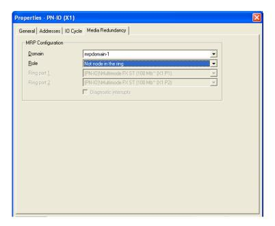
Figure 13: Dialog for entering the Media redundancy
