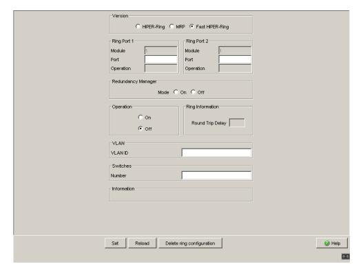
Figure 64: Selecting HIPER-Ring version, entering ring ports, enabling/disabling ring manager and selecting ring recovery
