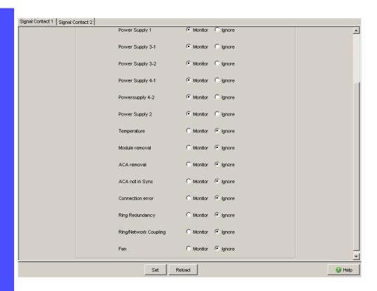
Figure 54: Monitoring the fan with the signal contact and trap
