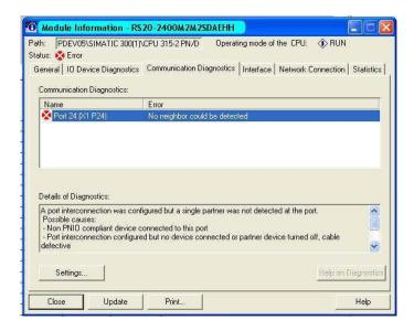
Figure 21: Diagnosis messages for the communication between the Switches and IO devices
