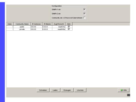
Figure 23: SNMPv1/v2 access dialog
