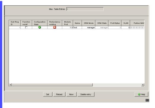
Figure 21: Completely configured Sub-Ring Manager
