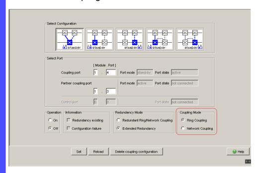
Figure 28: One-Switch coupling: Selecting the coupling mode
