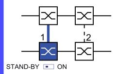
Figure 30: Two-Switch coupling
