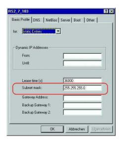
Figure 64: Netmask in the configuration profile
