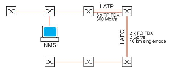
Figure 1: Example of link aggregation
