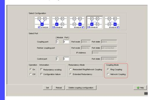
Figure 42: Two-Switch coupling with control line: Selecting the coupling mode
