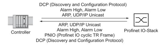
Figure 6: Communication between the Controller and the Switch
