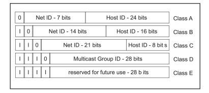
Figure 6: Bit representation of the IP address
