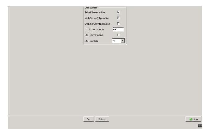
Figure 27: Telnet/Web/SSH Access dialog
