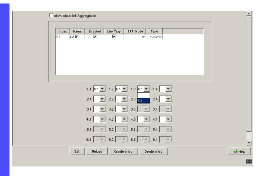
Figure 5: Assigning ports to link aggregation
