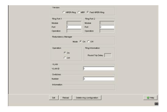
Figure 68: Selecting and configuring Fast HIPER-Ring
