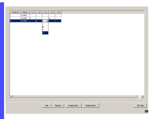
Figure 45: Defining the VLAN membership of the ports.
