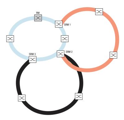
Figure 17: Special case: a Sub-Ring Manager manages 2 Sub-Rings (2 instances).
