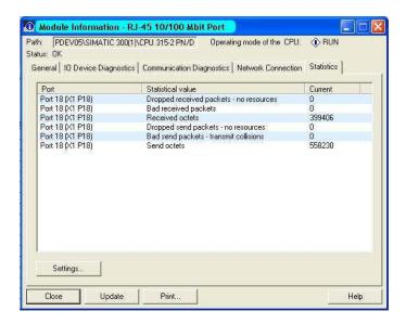
Figure 22: Example of a port statistic table
