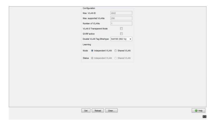
Figure 51: Switching: VLAN: Global dialog (MACH4000 and MACH 1040)
