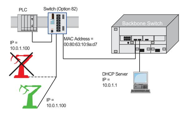
Figure 14: Application example of using Option 82
