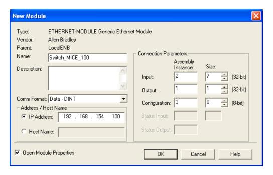
Figure 4: Integrating a new module into Logix 5000
