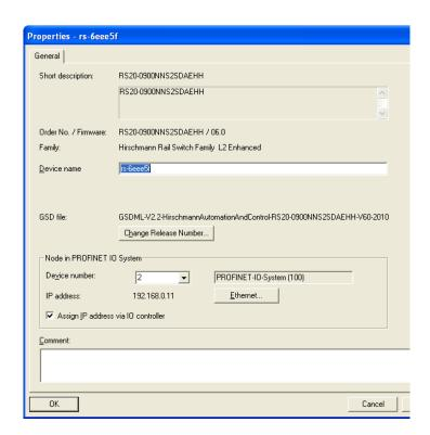
Figure 11: Dialog for entering the object name (= name of the Switch) and the IP parameter
