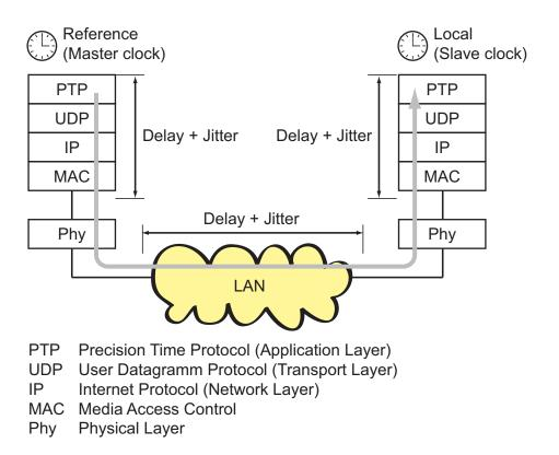
Figure 29: Delay and jitter for clock synchronization
