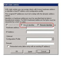
Figure 74: Default setting for the fixed address assignment
