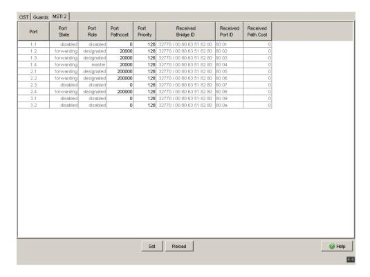
Figure 77: Multiple Spanning Tree dialog, Port, MSTI <ID> tab
