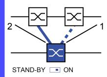
Figure 24: One-Switch-coupling
