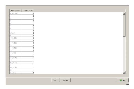
Figure 62: IP DSCP mapping table
