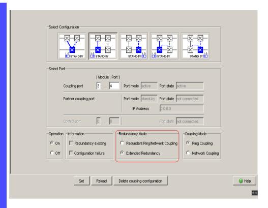
Figure 33: Two-Switch coupling: Selecting the redundancy mode
