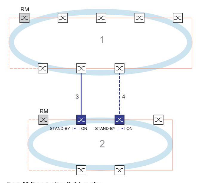
Figure 29: Example of two-Switch coupling
