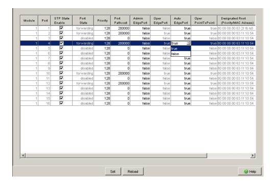
Figure 75: Multiple Spanning Tree dialog, Port, CIST tab
