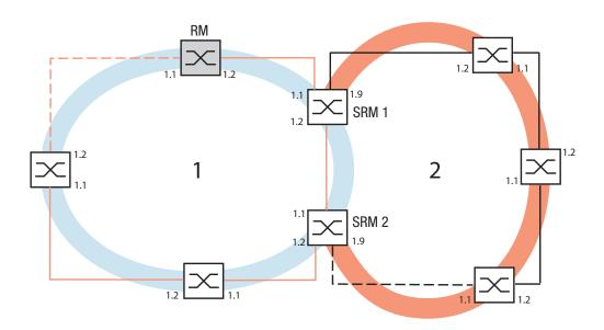
Figure 19: Example of a Sub-Ring structure
