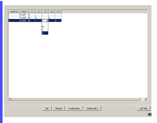
Figure 49: Defining the VLAN membership of the ports.
