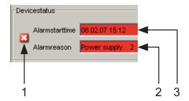
Figure 4: Device status and alarm display
