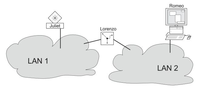
Figure 7: Management agent that is separated from its management station by a router
