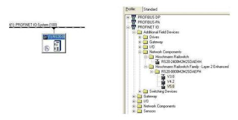
Figure 9: Adding a Switch from the Simatic S7 library
