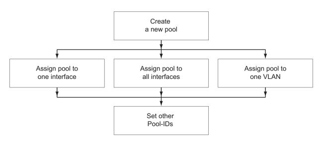
Figure 13: DHCP server: Create a pool per VLAN, or for one interface/all interfaces
