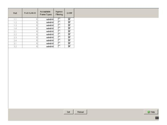
Figure 54: Switching: VLAN: Port dialog
