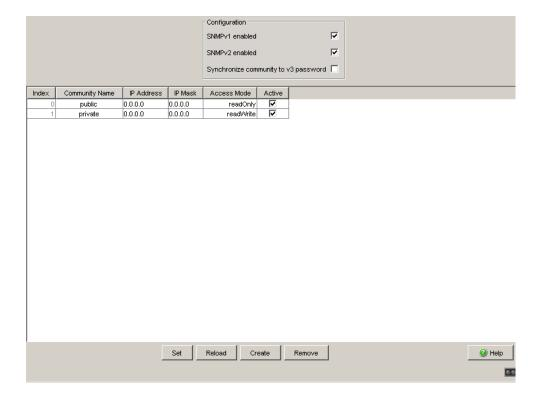
Figure 26: SNMPv1/v2 Access Dialog
