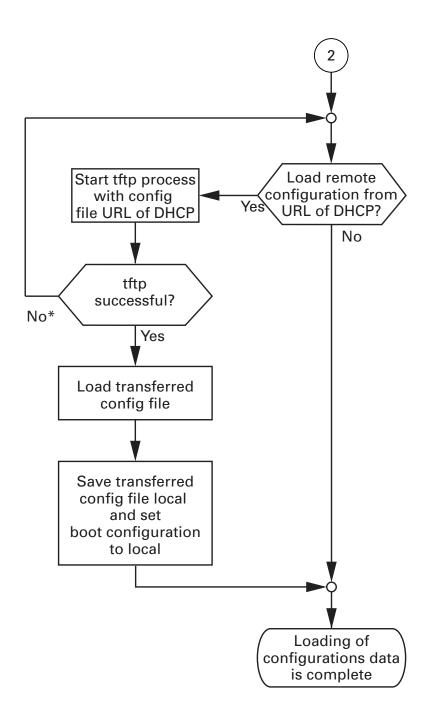
Figure 11: Flow chart for the BOOTP/DHCP process, part 2
