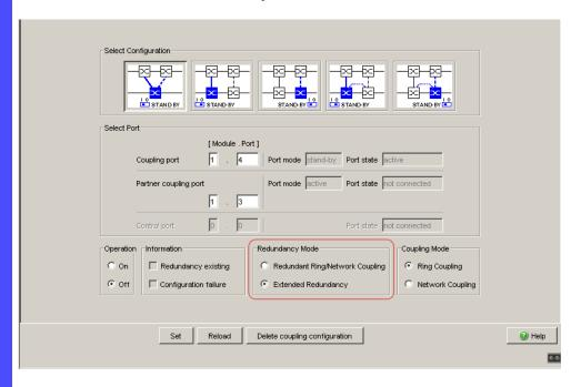
Figure 26: One-Switch coupling: Selecting the redundancy mode
