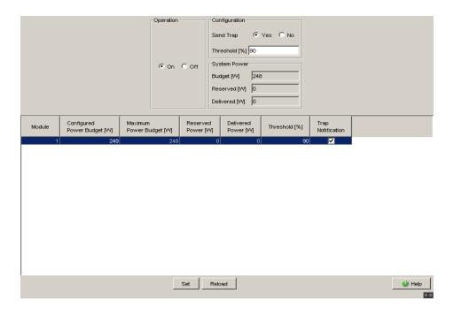
Figure 11: Power over Ethernet Plus Dialog:Global
