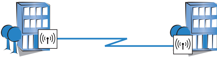
Figure 2: A wireless link between two access points
