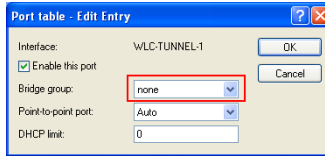
Figure 60: Port settings for public-spot APs
