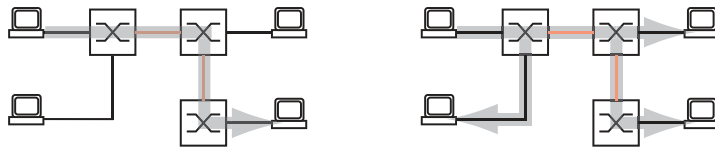
Figure 80: MAC Data Transmission: Unicast Data Packet (left) and Broadcast Data Packet (right)
