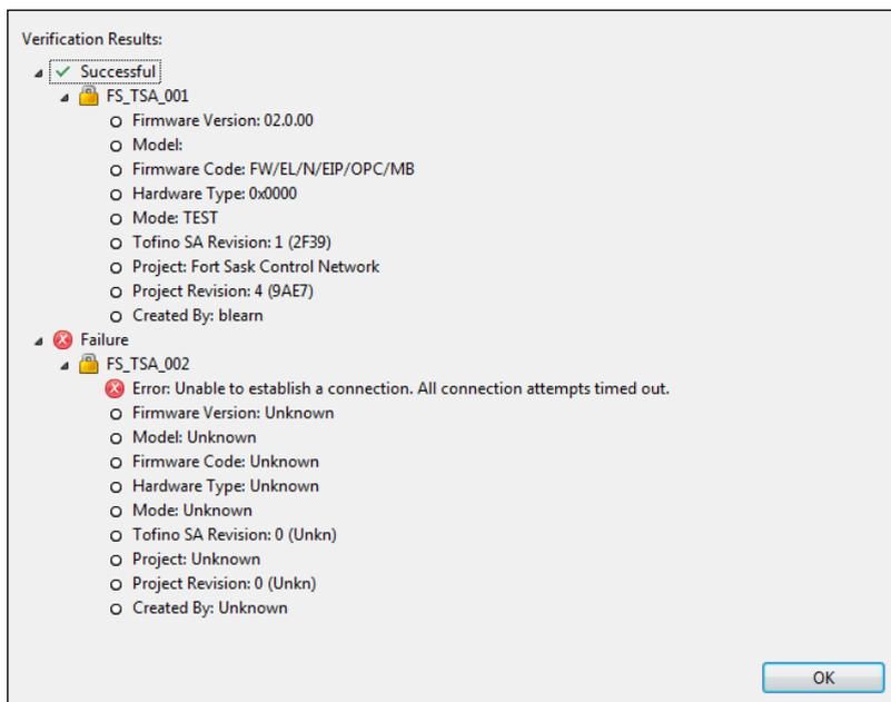
The Verified Configuration Revision, Hardware Type, and Firmware Version for the verified Tofino SAs will be updated in the project file. You can view the verification information on the General settings page for each Tofino SA.
